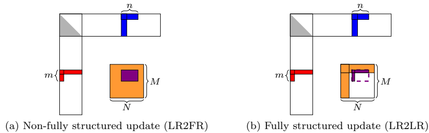
Figure 1: Representation of the updates, C -= AB , for the Just-In-Time strategy on the left, and Minimal Memory on the right. A appears in red, B in blue, C in orange, and the impact of the contribution AB in purple.
