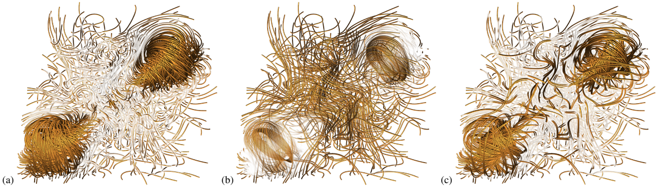
Figure 12: Opacity optimization results for different importance notions: (a) curvature; (b) linear entropy; and (c) point saliency.
