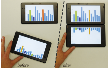
Figure 2: VisTiles [11] leverages multiple mobile devices for spatially-aware exploration of multivariate data.
