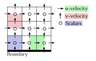
Figure 2. Sketch of the fully staggered mesh used for the space discretization.
