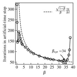
Figure 7. Unsteady cylinder wake (Mesh size of  $43 \times 246$ ): influence of the dimensionless artificial compressibility factor  $\beta$  on the number of time steps required to obtain an artificialtime converged solution. Comparison with the lower bound proposed by Chang and Kwak [6].
