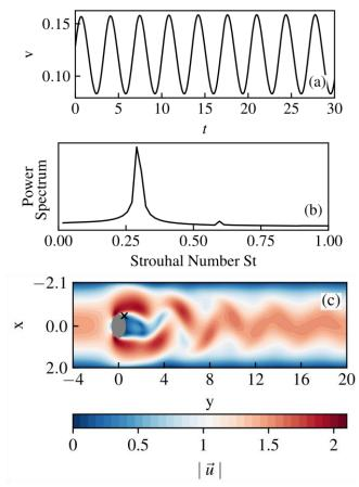
Figure 5. Unsteady cylinder wake (Mesh size of  $43 \times 246$ ): (a) Velocity history signal at (x, y) = (-0.5, 0.5), (b) Corresponding power spectrum of such velocity signal, and (c) Snapshot of the contour of the velocity norm (The marker × indicates the location at which the data in (a) are recorded).
