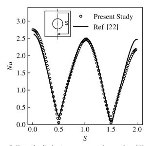
Figure 9. Heated cylinder in a square enclosure: Local Nusselt number distribution along the walls of the enclosure (Present results obtained with a grid resolution of  $101 \times 101$ ). Comparison with the numerical results of Kim et al. [22] obtained with a grid resolution of  $201 \times 201$ .
