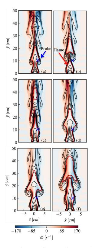
Figure 14. (a)  $\hat{t} = 1.3s$ , (b)  $\hat{t} = 1.35s$ , (c)  $\hat{t} = 1.39s$ , (d)  $\hat{t} = 1.43s$ , (e)  $\hat{t} = 1.47s$ , (f)  $\hat{t} = 1.52s$ . The red isoline represents the flame sheet (Z = 1) and the blue × marker represents the location of the probe from Figure 13a.
