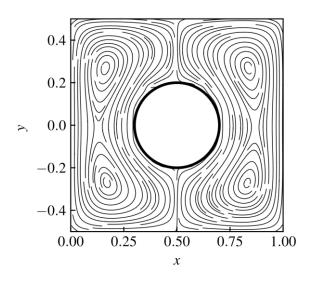
Figure 8. Heated cylinder in a square enclosure (Grid resolution of  $101 \times 101$ ): Streamlines patterns.
