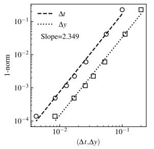
Figure 3. Physical time and spatial order of accuracy by the log-log scale analysis using 1-norm.
