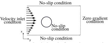
Figure 4. Unsteady cylinder wake: flow configuration and related boundary conditions.
