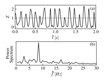
Figure 13. Flickering diffusion flame (Mesh size of  $41 \times 101$ ): (a) Mixture Fraction history at  $(\hat{x}, \hat{y}) = (1.3 \times 10^{-2}m, 10^{-1}m)$ , (b) power spectrum for the flame fluctuation.
