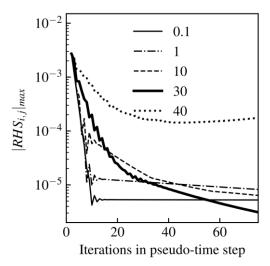
Figure 6. Unsteady cylinder wake (Mesh size of  $43 \times 246$ ): (a) Convergence history as a function of the dimensionless artificial compressibility factor  $\beta$ .
