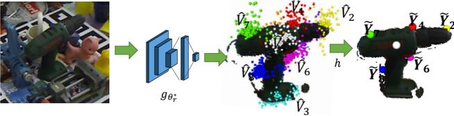
Fig. 5: Example of predicted 3D points. From left to right: the cropped input image, the cluster of 3D votes  $\hat{\mathbf{V}}_j$  where each color corresponds to votes for a single point, the aggregated points  $\tilde{\mathbf{Y}}_j$  obtained by mean-shift (best seen in color). The aggregated point of cluster  $\hat{\mathbf{V}}_3$  is hidden behind the driller point cloud.
