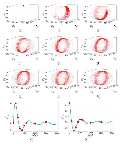
FIGURE 10. Full spin dependent model, with Dirac initial condition and  $v_{th}=0.51$ . Frames from (a) to (i): distribution of the spins on the unit sphere, at times  $\omega_p t=0,100,200,300,400,500,600,1000$ , and 1500. Frames (j) and (k) show time history of  $S_y(t)$  and  $S_z(t)$ , the red dots correspond to the times of the different snapshots displayed in (a)-(i).
