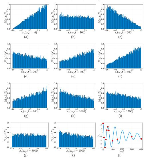
Full spin dependent model. Histograms of different  $s_z$ at $0.00022, v_{th}$  $0.17, \eta$ = 1. From case with h == (a)  $\omega_p t = 0,100,200,300,400,500,600,1000,1500,3000$ , and 4000.  $N(s_z)$  the number of particles having the z spin component in an interval around  $s_z$  and  $N_p$  is the total number of particles. The frame (l) shows the time history of the global spin component  $S_z(t)$ . The red dots corresponds to the times of the different histograms displayed in (a)-(k).
