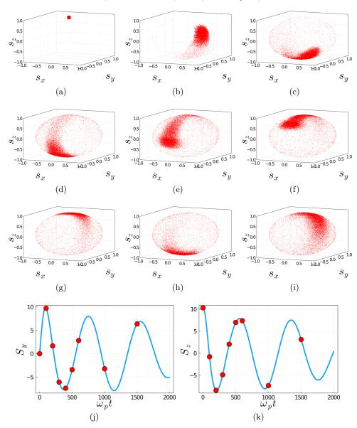
FIGURE 9. Full spin dependent model, with Dirac initial condition and  $v_{th}=0.17$ . Frames from (a) to (i): distribution of the spins on the unit sphere, at times  $\omega_p t=0,100,200,300,400,500,600,1000$ , and 1500. Frames (j) and (k) show time history of  $S_y(t)$  and  $S_z(t)$ , the red dots correspond to the times of the different snapshots displayed in (a)-(i).
