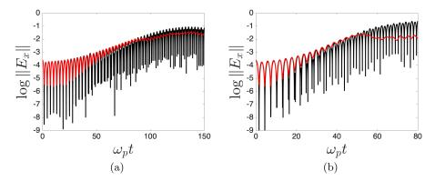
FIGURE 2. SRS simulations without spin. Time evolution of the amplitude of the longitudinal electric field norm  $||E_x(t)||$  on a semi-log<sub>e</sub> scale. We compare the results of the Eulerian grid code (black curves) and the PIC code (red curves), for two values of the initial amplitude of the electromagnetic wave. Left frame:  $E_0 = E_{\rm ref} = 0.325$  (observed slope in the linear regime:  $\gamma \approx 0.03$ ). Right frame:  $E_0 = 2E_{\rm ref} = 0.65$  ( $\gamma \approx 0.06$ ).
