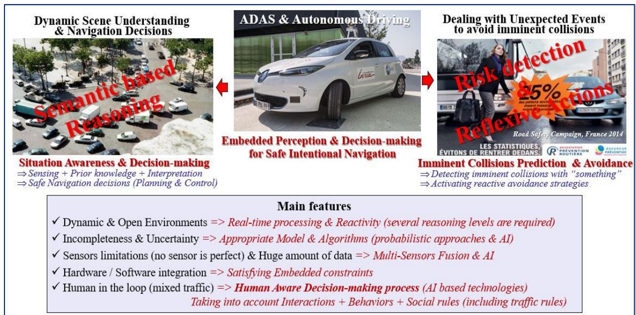
Figure 1: Illustration of our approach for addressing the problem of Embedded Perception & Decision-making for Autonomous Vehicles (by mixing Bayesian & AI approaches)
