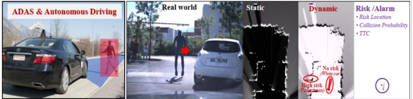
Figure 7: Illustration of the concept of “Bayesian Short-term Collision Risk” implemented in the CMCDOT system [23, 25]. The approach combines our “Conservative short-term Motion Prediction model” (horizon 3-5 seconds), with a probabilistic estimation of the Collision Risks.
