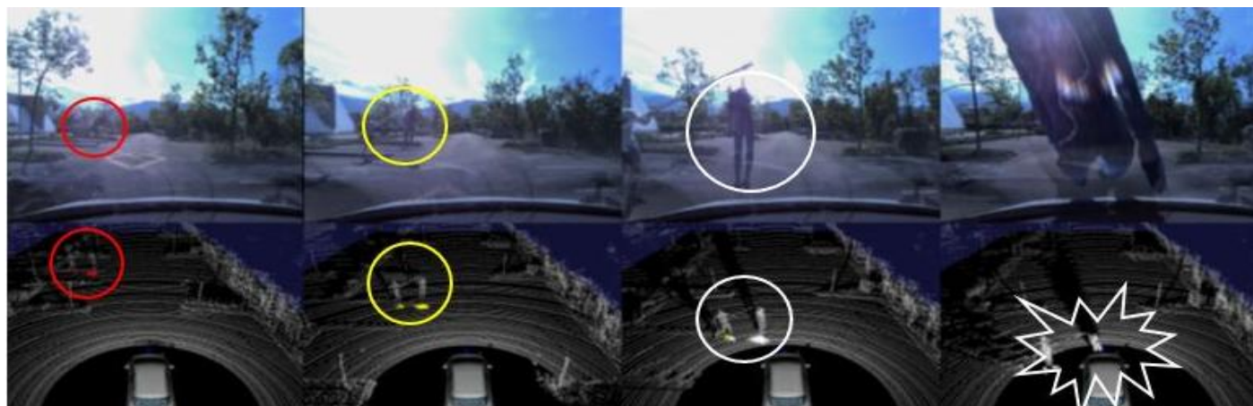
Figure 10: Illustration of one of the experiments performed with Inria’s autonomous car. The scenario reproduces the car colliding with a pedestrian (mannequin) crossing the street [52].
