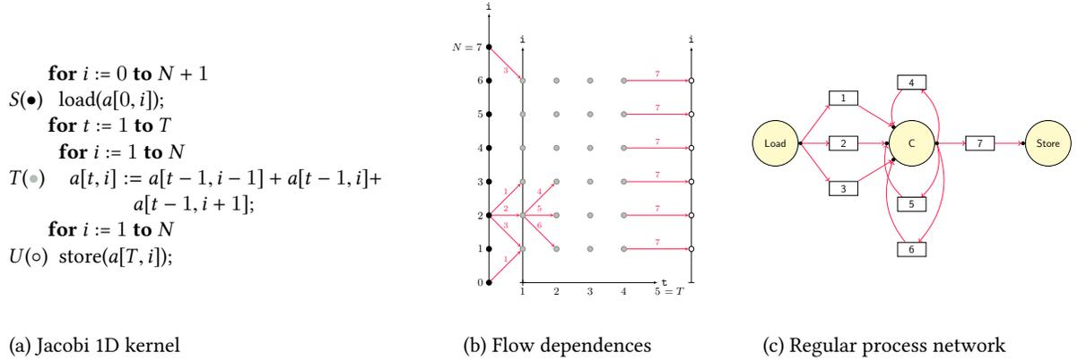
**Figure 1.** Motivating example: Jacobi-1D kernel. (a) depicts a polyhedral kernel, (b) gives the polyhedral representation of loop iterations ( $\bullet$ : load,  $\circ$ : compute,  $\circ$ : store) and flow dependences (red arrows), then (c) gives a possible implementation as a regular process network: each assignment (load, compute, store) is mapped to a different process and flow dependences (1 to 7) are solved through channels.
