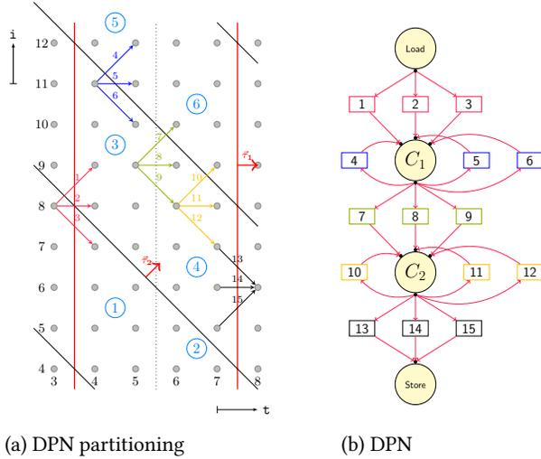
**Figure 2. Data-aware process network (DPN) for the Jacobi-1D kernel.** (a) computations are executed per band (between red thick lines), tile per tile. Incoming dependences (1,2,3) are loaded, outgoing dependences (13,14,15) are stored, internal dependences (4 to 12) are solved through local channels depicted in (b). Parallelization is derived by splitting a band with outer tiling hyperplanes (here the dotted line). With this scheme, arithmetic intensity and parallelism can be tuned easily.
