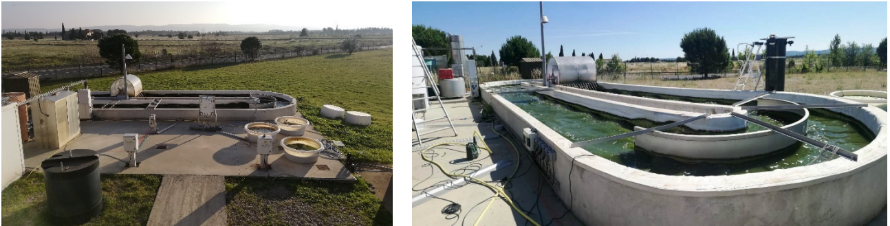
Figure SI.1.1. demonstrative scale raceway (17 m 3 ), located in Narbonne, France (INRAE).
