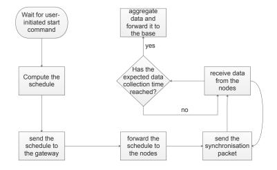
Fig. 8. Experimental procedure of Base/Gateway.
