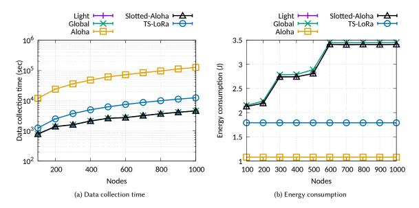
Fig. 5. Data collection time and energy consumption for a scenario with fixed data size.
