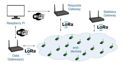
Fig. 9. Network architecture of the experiments.
