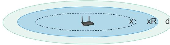
Fig. 1. Interfering zone (dark colour) of a node located at distance  $x$  from the gateway placed at the center of the disk (intra-SF interference).
