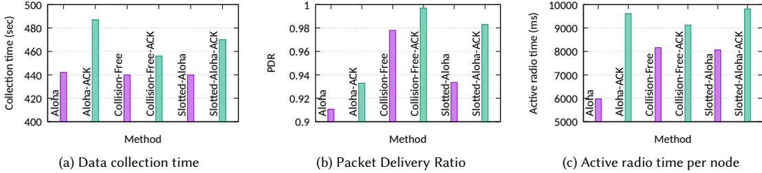
Fig. 10. Experiment with 10 nodes: Data collection time, Packet Delivery Ratio, and active radio time with and without retransmissions (CF: Collision-Free approaches, S-Aloha: Slotted-Aloha, -ACK: the corresponding approach with retransmissions).
