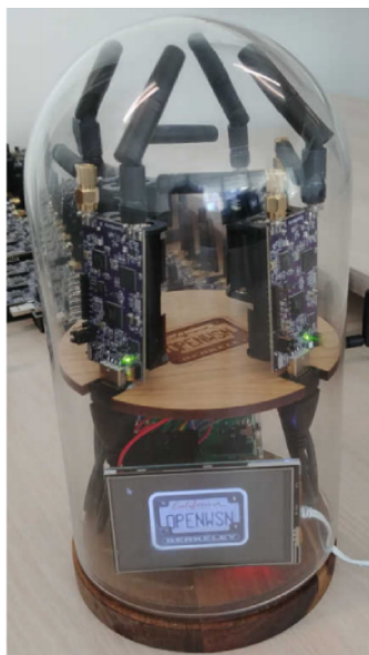
FIGURE 3 – The OpenTestbox used for experimental evaluation in the Open Testbed. Borrowed from [12].
