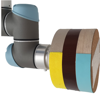
Fig. 3. The designed cylindrical prop for representing our approach. This prop can hold different textures which are used to render flat surface in a VE. Textures as cork, foam, felt, leather, cardboard and wood are displayed on this figure. In this case, the leather texture covers the prop's whole circumference, this permits to render this texture in an infinite way as long as the prop spins below users' finger.
