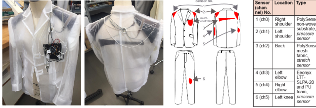
Figure 6: Jacket part of tailored interactive suit, and sensor distribution.
