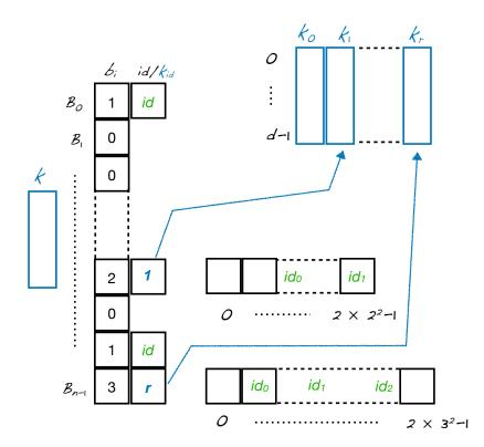
Figure 1 – In the proposed variant of FKS, for each bucket  $B_i$ , we store the number  $b_i$  of hyperedges assigned to  $B_i$ . If  $b_i$  is 0, nothing else is stored for  $B_i$ . If  $b_i$  is 1, the id of the hyperedge mapping to i is stored. If  $b_i$  is larger than 1, then the index of a suitable *d*-tuple from  $\mathbf{k}_0$  to  $\mathbf{k}_r$  in K is stored, along with a space of size  $2b_i^2$  to hold the ids of  $b_i$  hyperedges assigned to  $B_i$ .
