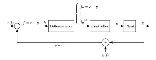
Figure 1: A typical control loop
