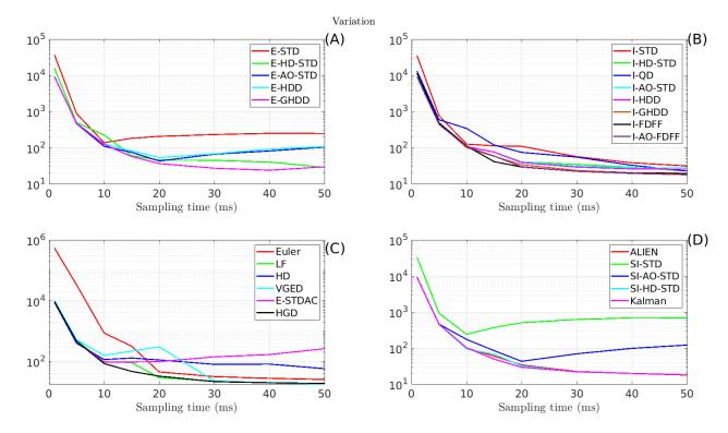
Figure 5: Variation of the control signal u(t) under different sampling times
