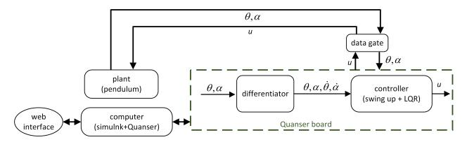
Figure 10: Closed-loop diagram of the RIPS
