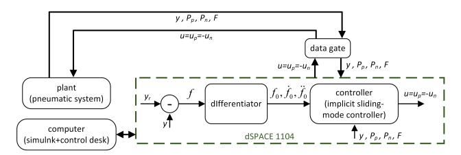
Figure 3: Closed-loop diagram of the EPS
