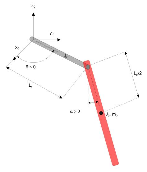
Figure 9: Scheme of the rotary inverted pendulum [1]
