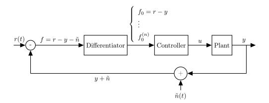
Figure 1: A typical control loop
