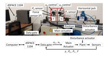
Figure 2: Electropneumatic setup
