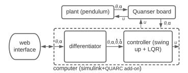
Figure 10: Closed-loop diagram of the RIPS
