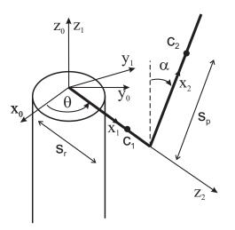
Figure 9: Scheme of the rotary inverted pendulum
