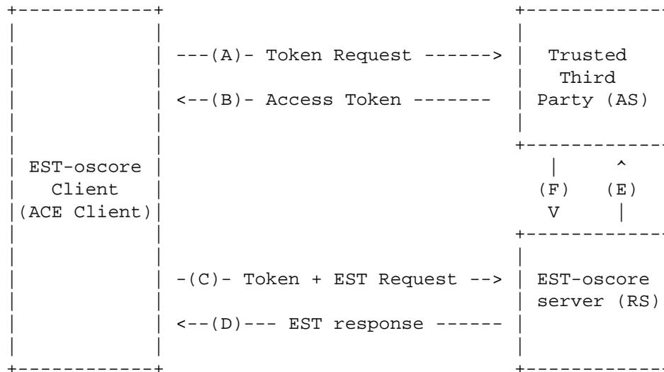
Figure 3: Accessing EST services using a TTP for authenticated key establishment and authorization.
