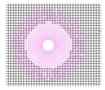
Fig. 1: Example of Chimera grid configuration. In black there is the background mesh and in blue the foreground mesh.
