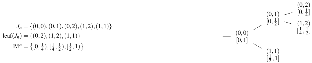
Fig. 6 Example tree representation of 1D wavelets. Left: nodes, leaves, and mesh of discretisation. Right: arrangement into a tree with index (j,k) and corresponding support of wavelet w_{j,k} underneath.
