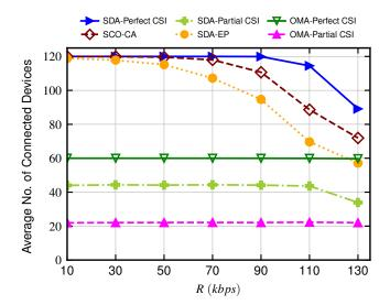
Fig. 8. Connectivity performance with varying service rate and M = 2 for 5 PRBs.
