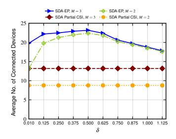
Fig. 1. Effect of  $\delta$  on the number of connected devices through SDA-EP based on (15).
