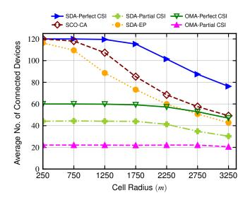
Fig. 12. Effect of cell radius on the connectivity performance of various algorithms with M = 2.
