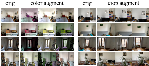
Fig. 3. Illustration of data augmentation that we use to train our model. We consider both color jittering (left) and random crops (right). For a panoramic observation with v views, the parameters of the augmentation are sampled independently.
