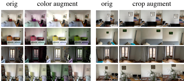
Figure 3. Illustration of data augmentation that we use to train our model. We consider both color jittering (left) and random crops (right). For a panoramic observation with v views, the parameters of the augmentation are sampled independently.
