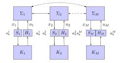
Fig. 4. A decentralized controller setup example.  $S_i$  and  $H_i$ , for all  $i \in \{1, 2, ..., M\}$ , denotes the sample and hold components, respectively, for the  $i^{th}$  closed-loop.
