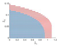
Fig. 9. Feasible values of  $\bar{h}_1$  and  $\bar{h}_2$ , when  $\bar{\eta}_1 = \bar{\eta}_2 = 0.075$ , for the large-delay case (in blue) and the small-delay case (in red). For the small-delay case, the bounds  $\bar{h}_1 < 0.075$  and  $\bar{h}_2 < 0.075$  are applicable only if the condition (70) is satisfied.
