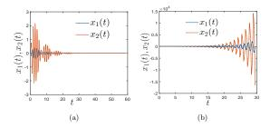
Fig. 1. (a) The decentralized LTI system (1) is stable for synchronous sampling with T = 0.59. (b) Stability is lost when  $x_2(t)$  is sampled asynchronously with respect to  $x_1(t)$  with a shift of  $\delta = 0.2$ .
