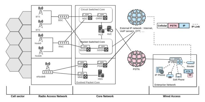
Fig. 2. Telephony networks architecture overview : Cellular network, PSTN network, VoIP network and gateways; from the access to the core.
