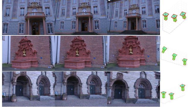
Figure 9. Trifocal relative pose estimation of EPFL dataset. For each row, image triplets samples are shown. The estimation results are shown on the right. Ground truth poses are in solid green and estimated poses are in red. More examples in supplementary material.
