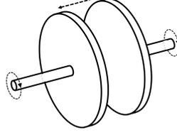
Figure 1: An ideal clutch with two shafts.
