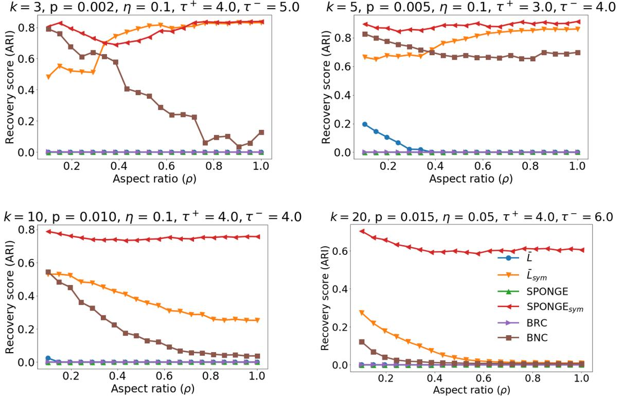
Figure 3: Performance of the various clustering algorithms, as measured by the Adjusted Rand Index, versus the aspect ratio  $\rho$  for a SSBM with  $k = \{3, 5, 10, 20\}$  for  $n = 5000$ . For larger number of clusters,  $k = 10$  and especially  $k = 20$ ,  $\text{SPONGE}_{sym}$  is essentially the only algorithm able to produce meaningful results, and clearly outperforms all the other methods. Note that no regularization has been used throughout this set of experiments.
