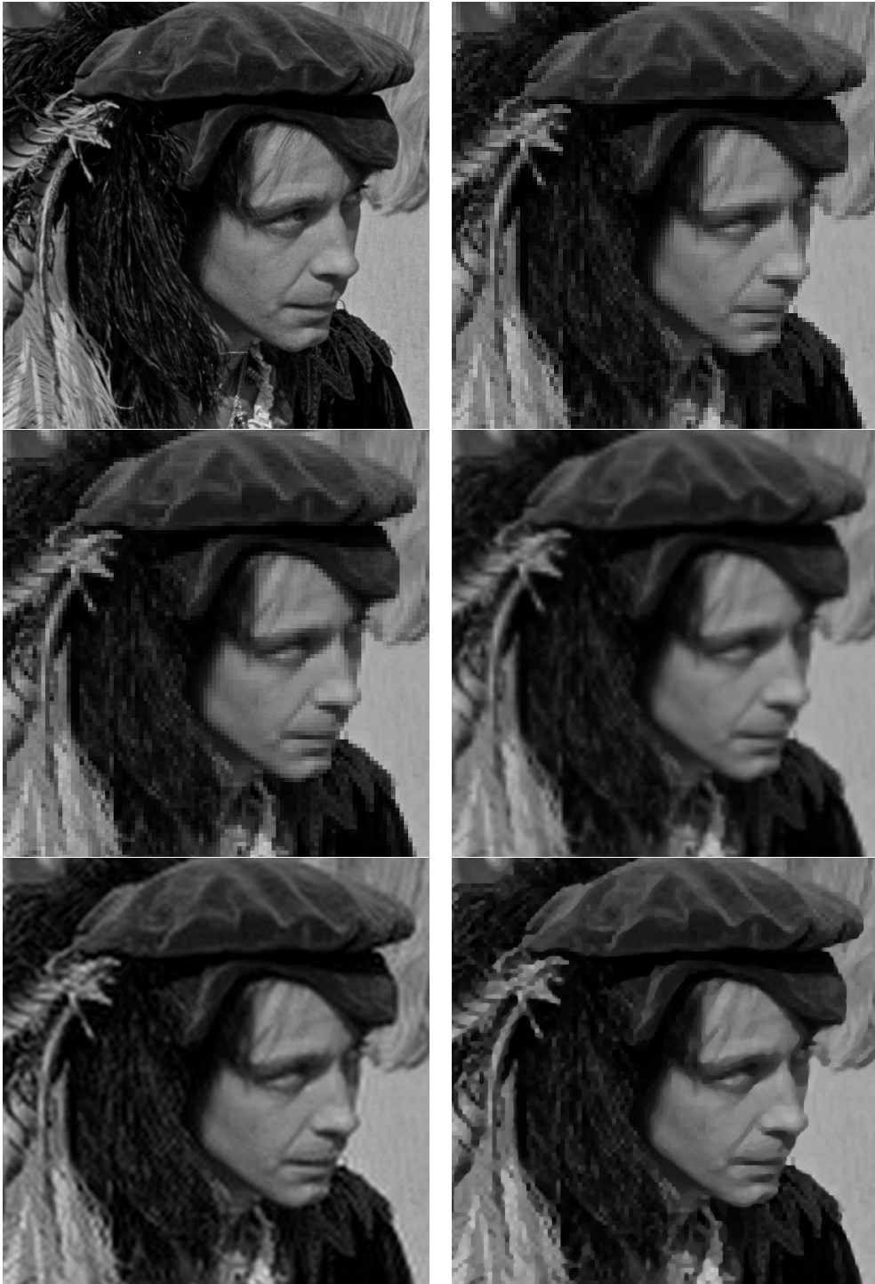
FIG. 6 – Image upsampling experiment. From left to right and top to bottom : original image (1024x1024), image convoluted, downsampled by 4 in each directions with an additive Gaussian noise, nearest neighbor interpolation (14.5 dB), bilinear interpolation (SNR 15.4dB), sinus cardinal interpolation (19 dB), TV-l^2 (SNR 19.7dB, 20 seconds).
