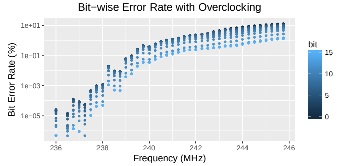
Fig. 12. Observed bit-wise error rate in the outputs with 16 \times 16 bits design, with uniform random inputs.
