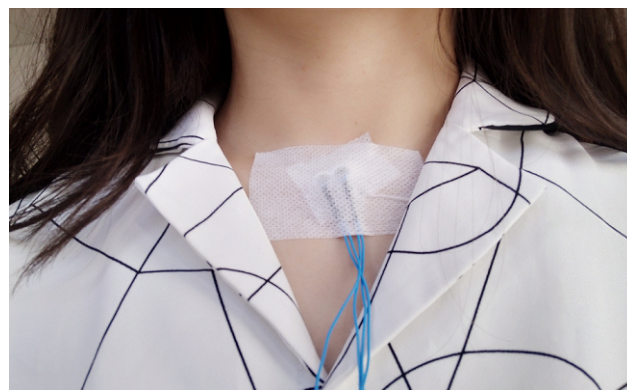
Figure 2. Position of the microphones: two microphones are inserted into the support that is fixed at suprasternal notch with two strips of adhesive tape.
