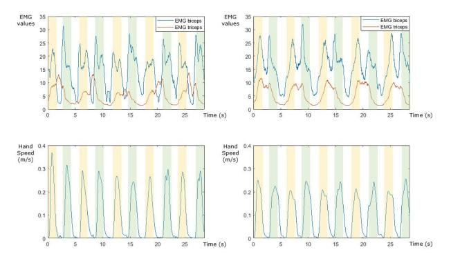
Fig. 5. Averaged EMG data (top) and hand speed (bottom) for real task (real visual feedback and haptic interaction) (left) and for virtual task (virtual visual feed back and synthetic haptic interaction) (right) at low speed. Yellow zone: outward phase, green zone: return phase, white zone: rest phase.
