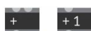
Figure 1 Gen example: the “+” function has two inlets by default, one will be suppressed by adding an argument
