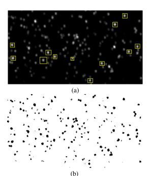
**Fig. 2**. Image depicting beads of 100 nm diameter used for resolution measurement. (a)  $I_{pc}(x)$  image with squares showing regions used to select 12 beads for measurement. (b) Binary image of Otsu threshold on  $I_1(x)$ .
