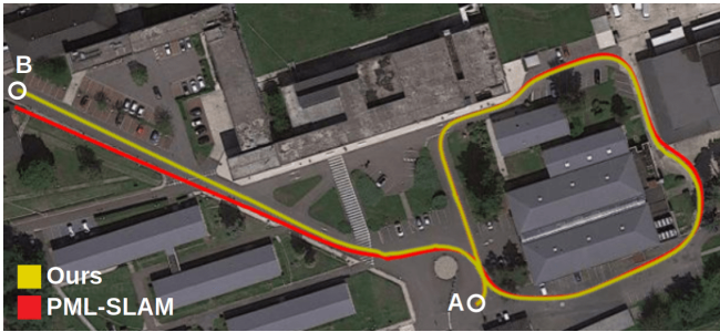
Fig. 4. Estimated trajectories from our method (yellow) and PML-SLAM (red) overlaid on google maps satellite images for the campus-A sequence. The trajectory starts in the area denoted A and ends in the area denoted B.
