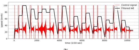
**Figure 3.** Representation of the performance of IAE optimized controller, with the system output unfiltered (**a**) and filtered (**b**).
