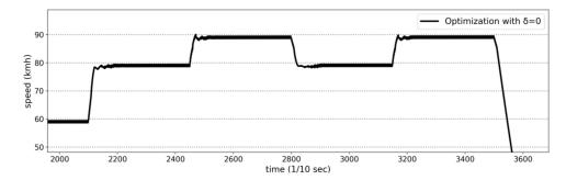
**Figure 7.** Detail of some step responses disabling the decay ratio d ( $\delta = 0$ ), clearly showing the oscillations in the controller performance.
