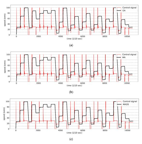
Figure 4. Representation of the performance of GA (a), MA (b) and MADS (c) optimized controllers.
