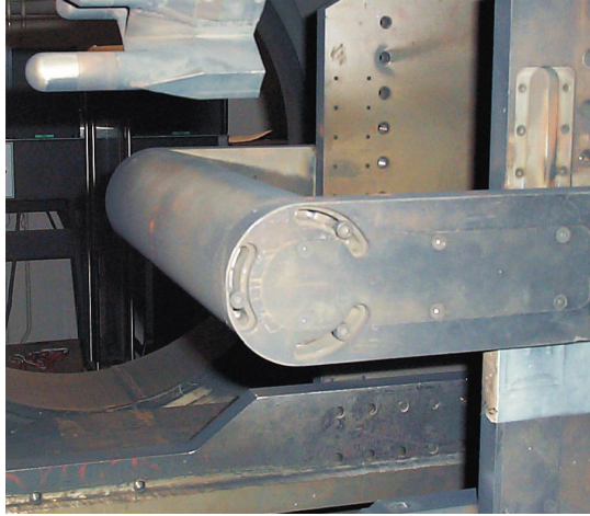
Figure 2: Image of the cylindrical experimental model in the HEG facility (taken from [11]).
