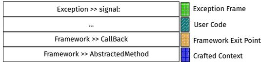
**Figure 4.** Representation of a call stack, with a crafted context inserted before the framework exit point.
