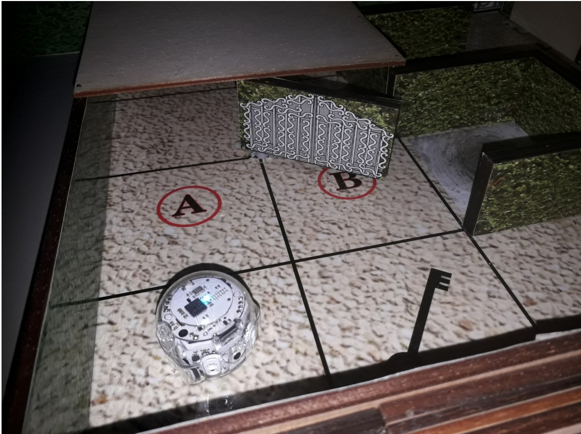
Fig 3B. The view of the conditional part of the path. A door can either obstruct the A gate or the B gate. Thus, optionally, beyond a simple instruction sequence, a programming gate can randomly either open the A or B passage. If the A or B state is known before the robot starts, this only involves modifying the instruction sequence. If this state changes after the robot starts moving, this involves using a conditional expression, as shown on the right.
