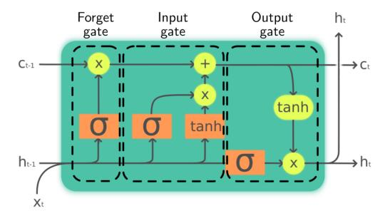
Figure 2: Architecture of one LSTM cell. A LSTM is composed of special cells  $c_t$  that keeps relevant features and the hidden state vector  $h_t$  that output information towards other recurrent cells and the output layer. Three gates are used to decide which information to store in the cell, to forget or what to output.
