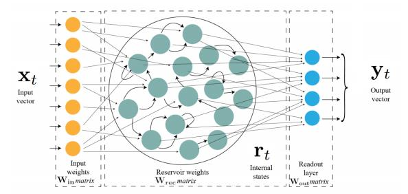
Figure 1: The ESN is trained to extract the target activation from the dynamic of the reservoir. To do this, only the readout connections, i.e. the coefficient of the matrix  $\mathbf{W_{out}}$ , are trained. This image was adapted from [39] with the authorisation of the authors.
