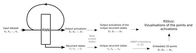
Figure 10: Protocol to create RSSviz. We used only unique recurrent states to avoid a resultant space distorted toward states that appears with high frequency.
