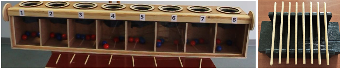
Fig. 3. Left: This “AI” machine is made of “balls and bowls” (or any equivalent objects) and after training will always win the “nim game”, just putting for each move a red or blue ball, depending on the game issue (win or lose), in the bowl corresponding to each move. After training the whole game policy is stored in the “machine” and the artificial player just has to choose what to play counting the balls in the corresponding bowl. Right: The “Nim game” is a simple strategy game in which two players (here a human and the “machine”) take turns removing (or “nimming”) objects 1, 2 or 3 objects (here rods), the loser making the last nimming. This setup allows us to understand what is an algorithm (including algorithmic recursivity), what is called “reinforcement learning”, why a mechanism can “learn” a non-trivial rule (in fact, “always leaving a multiple of 4 rods”), without understanding anything. Images from https://pixees.fr as open CC-BY resources.
