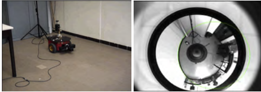
Fig. 4. Navigation of a mobile robot to follow a wall using an omnidirectional vision sensor. The 3D straight line at the bottom of the wall projects as a circle in the image (depicted in green). This circle does not move if the robot follows the wall while it moves if the robot is not correctly oriented.
