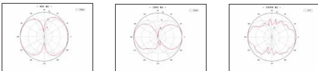
Figure 7b. Reproduction de H1 @ 500 Hz, 2000Hz & 10000 Hz
