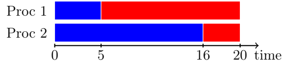
Figure 1: Toy example with two processors, two successfully completed tasks (in blue) and two not-yet-completed tasks (in red) at time 20.
