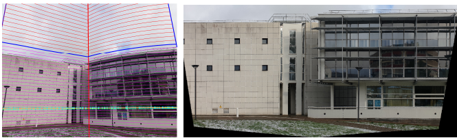
Fig. 9. An example of result obtained with our method as it stands on an image of a building, demonstrating the genericity of our approach. Left: Acquired image with graphic layers showing the intermediate results of the algorithm. Right: Dewarped building.
