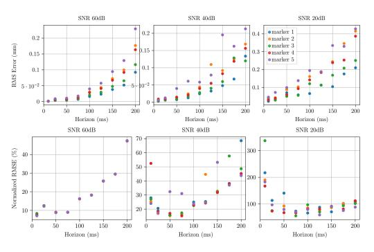
Figure 5.6: Second order Linear prediction filter performance over simulation data for 60dB, 40dB and 20dB SNR. An optimal regression window was used for each signal as described in section 4.1.4.
