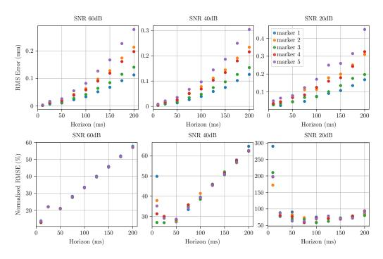
Figure 5.5: First order Linear prediction filter performance over simulation data for 60dB, 40dB and 20dB SNR. An optimal regression window was used for each signal as described in section 4.1.4.
