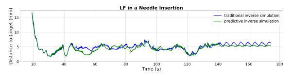
Figure 5.9: Motion compensation distance to target comparison between predictive inverse simulation and traditional inverse simulation. This corresponds to the objective function  $\mathbf{e}_p$  of the inverse simulation control framework. This metric was measured from the direct simulation with a rigid needle with 200*GPa* Young Modulus.
