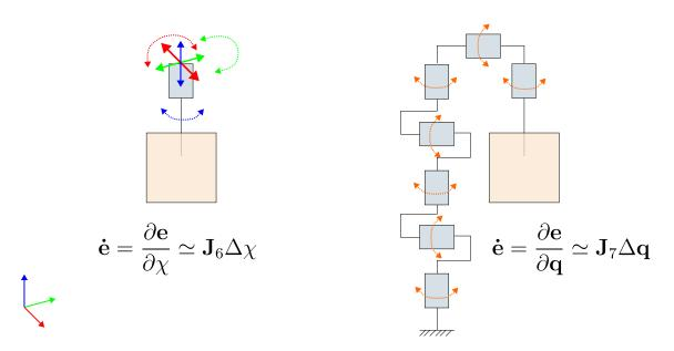
Figure A.1: Finite differences method applied to a needle insertion robot end effector and to each of the robot's joints, on the left and right sides respectively. The first derivative of the objective constraints for this configuration  $\dot{\mathbf{e}}$  is related to the end effector position though the Jacobian matrix  $\mathbf{J}_6$ . Similarly,  $\dot{\mathbf{e}}$  is related to the robot joint positions through the Jacobian matrix  $\mathbf{J}_7$
