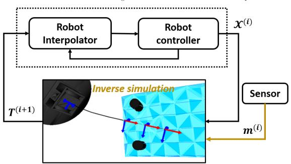
Figure 3.1: Adapted from [2], expresses the inverse simulation as the feedback loop to derive robotic commands for the needle steering. The robot interpolator and robot controller are assumed to be embedded into the robot's controller architecture.
