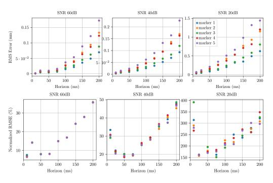
Figure 5.4: Second order Linear prediction filter performance over simulation data for 60dB, 40dB and 20dB SNR. A fixed regression window of 10 samples was used for both filters.
