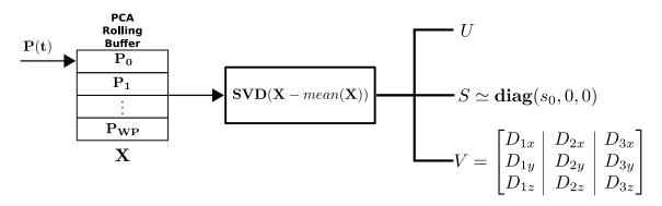
Figure 4.1: Preparation phase for the linear prediction filter. A rolling buffer of size WP stores the Cartesian position of each marker on the previous time steps  $P_i, i \in [0, WP]$ . An singular value decomposition (SVD) is applied to the centered rolling buffer and the first singular value usually overweighs the remaining values [49]. The principal components of the signal are the columns of the V matrix [51].
