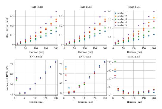
Figure 5.3: First order Linear prediction filter performance over simulation data for 60dB, 40dB and 20dB SNR. A fixed regression window of 10 samples was used for both filters.
