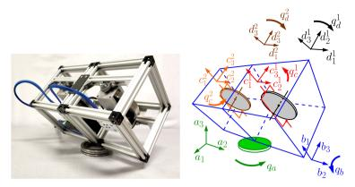
Fig. 2. Left: inverted pendulum hardware that we study in this paper. The pendulum consists of six bodies: body *A* (the thrust bearing), body *B* (the frame), bodies  $C^1$  and  $C^2$  (the single-axis gimbals), and, finally, bodies  $D^1$  and  $D^2$  (the flywheels). **Right:** corresponding notations. This configuration corresponds to  $q_b = -\pi/4$  and  $q_c^1 = q_c^2 = \pi/2$ .
