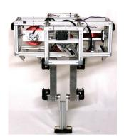
Fig. 1. We are developing a biped that uses four control moment gyroscopes (highlited in red) as an auxiliary stabilization system.
