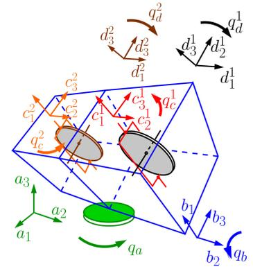
Fig. 2. **Left:** inverted pendulum hardware that we study in this paper. The pendulum consists of six bodies: body  $A$  (the thrust bearing), body  $B$  (the frame), bodies  $C^1$  and  $C^2$  (the single-axis gimbals), and, finally, bodies  $D^1$  and  $D^2$  (the flywheels). **Right:** corresponding notations. This configuration corresponds to  $q_b = -\pi/4$  and  $q_c^1 = q_c^2 = \pi/2$ .
