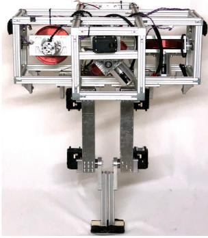
Fig. 1. We are developing a biped that uses four control moment gyroscopes (highlited in red) as an auxiliary stabilization system.
