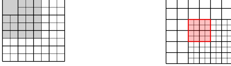
Figure 2: Left: Support of a cubic HB-spline (entire box) and of a THB-spline (grey) of level 0 on a hierarchy with two levels, N = 1 . The associated coefficient functional is supported on the larger cell (that belongs to \Omega^0 \setminus \Omega^1 ) in the top left corner. Right: Hierarchy of 2 levels \Omega^0 and \Omega^1 , subdomain \Delta = \hat{\Omega}^0 highlighted in red. We have \hat{\Omega}^0 = \Omega^1 , hence \hat{J}^0 = \emptyset and \hat{J}^1 \not\subseteq J^1 .
